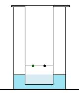
Place small a spot of the mixture to be analysed (and any possible component for comparison purposes) on the paper. Dip the paper in the solvent.
