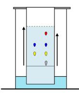
Allow the solvent to rise up the paper. Each component dissolves in the solvent. Those which are more soluble travel further up the paper.
